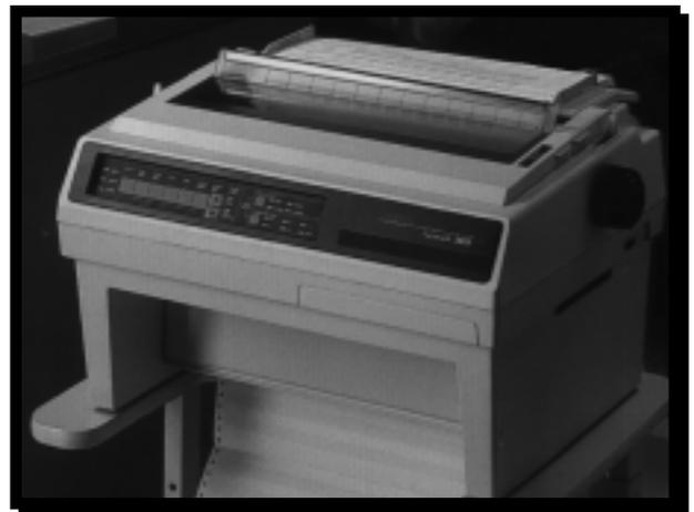
**2550** *Dot Matrix printer***TYPE**9 pin dot matrix
